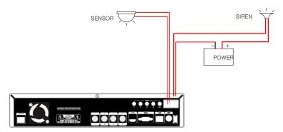
**Sensor In**: Connect the sensors. The sensor are composed of both signal and ground terminals, with a voltage difference of 5V. In the case that the sensor used for input is of the N/O (Normal Open) type, when the voltage difference between the signal and ground falls to 0V (short), the DVR can use this as a trigger to start alarm/sensor based recording.
