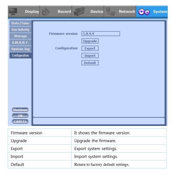
You should connect correctly the USB devices, before you use firmware upgrade, export and import.
