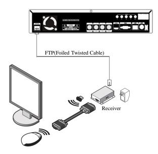
2. Because all the case has different cable length, you should adjust the GAIN and PHASE in Receiver to get a most proper VGA output. You can use the small cross screw driver for adjusting at the edge of Receiver.
