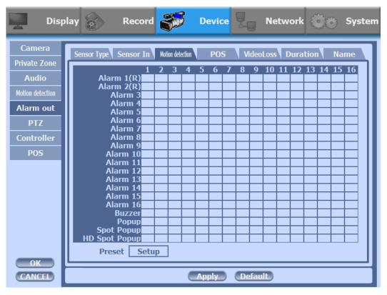
• Also you can choose more than one action. Furthermore you can set the preset position number by motion detection. If you push the 'setup' you can see the preset screen.
