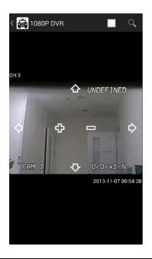
If the PTZ camera is set on the DVR, PTZ button will appear automatically and allow you to control PTZ camera.
